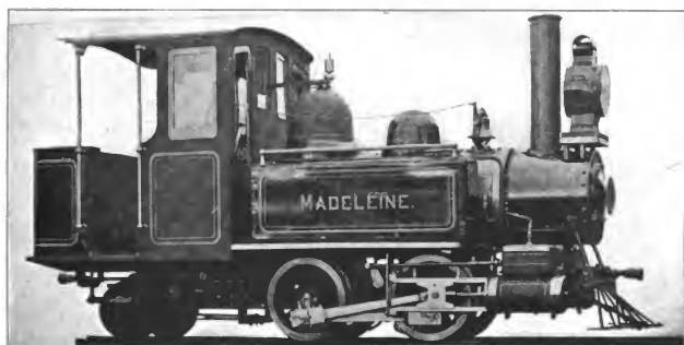
Fig. 10. Four-Coupled (0-4-2) Tank Locomotive with Trailing Truck. Built by the American Locomotive Co. Cylinders 8 in. x 12 in., Working Steam Pressure 180 lbs. per sq. in., Heating Surface 226 sq. ft., Diameter of Drivers 28 in., Weight on Drivers 17,600 lbs., Total Weight 20,300 lbs.
